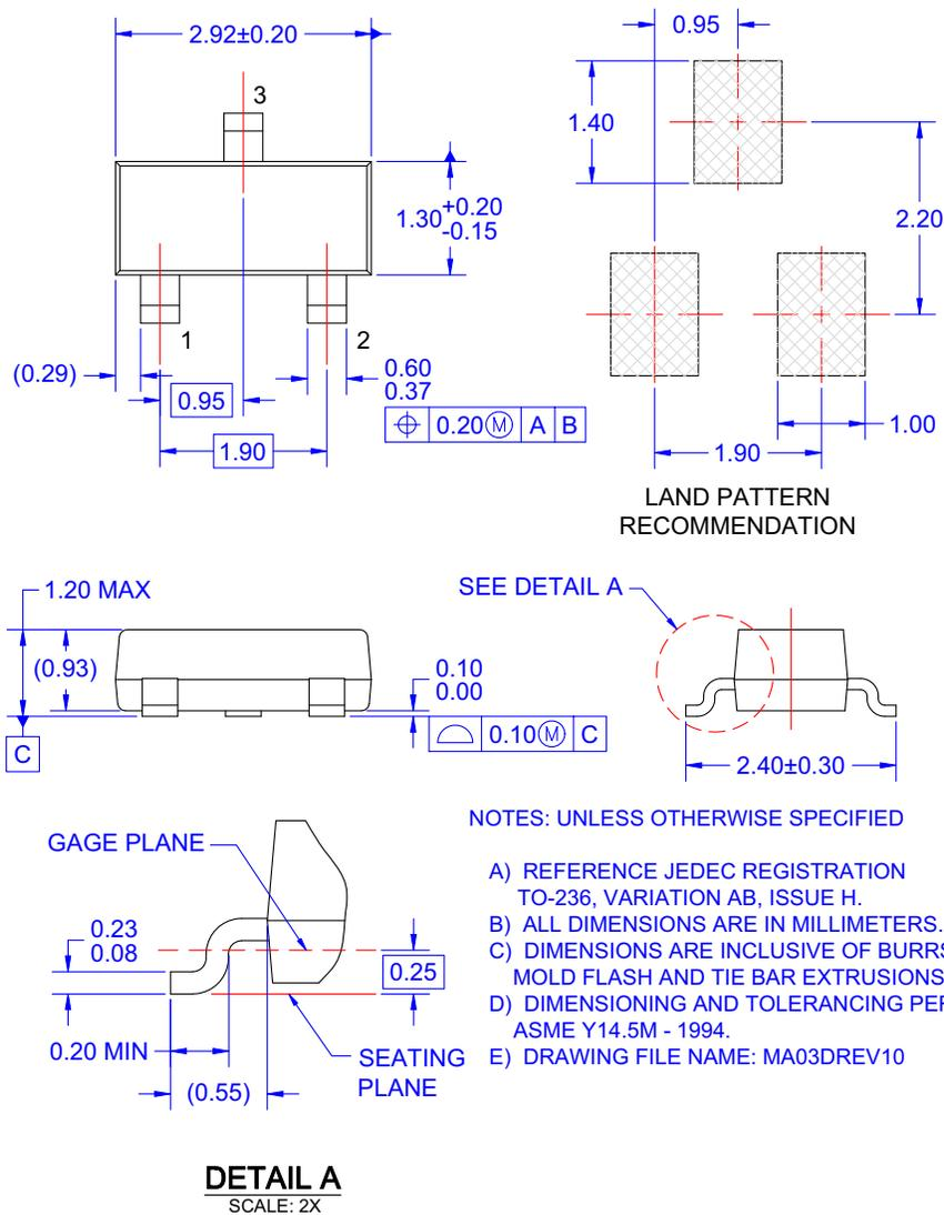
Figure 16. 3-LEAD, SOT23, JEDEC TO-236, LOW PROFILE (ACTIVE)
